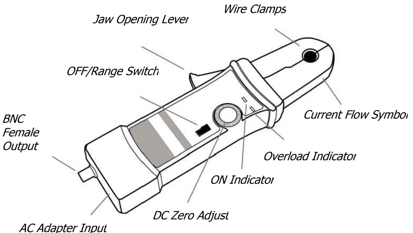
**Figure 1:** Controls and indicators on current probe
