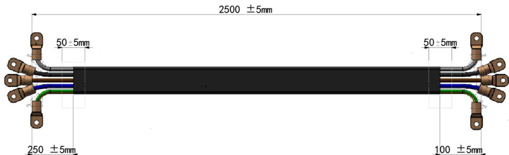
Connect the five terminals brown to line (L1), gray to line (L2), black to line (L3), blue to neutral (N), and yellow-green to ground (PE) on the other end of the power cord to your AC distribution panel.
