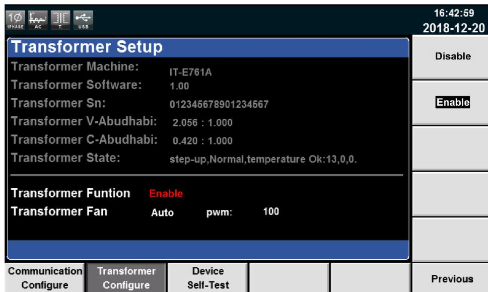
4. Press **[Enable]** to turn the transformer function on.
