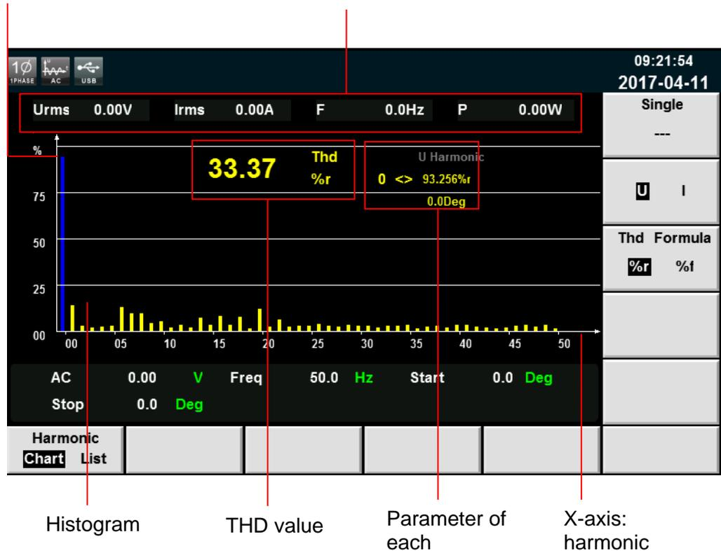
Total harmonic parameters: Under single phase mode, display total harmonic distortion of the single phase. Under three-phase mode, display total harmonic distortion (THD) factors corresponding to Phase A, B and C.
