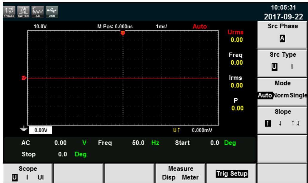
3. Press the soft key corresponding to the parameter on the right side and select the required trigger configuration.
