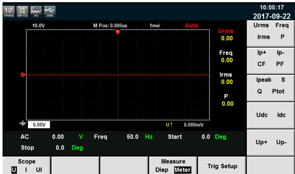
3. Press soft keys on the front panel to select the measuring parameters you need.
