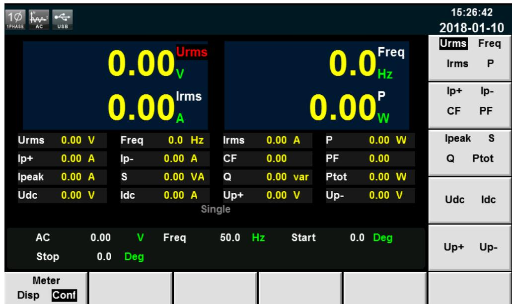
The user can self-define the screen parameters. Four large-font parameters are displayed on the upper part of the interface. The above figure shows the voltage, frequency, current and active power. Press the Up and Down keys to move the cursor, and select the parameter (red background). Press the corresponding soft key on the right side to adjust the current parameter. Set all the parameters by the above steps.
