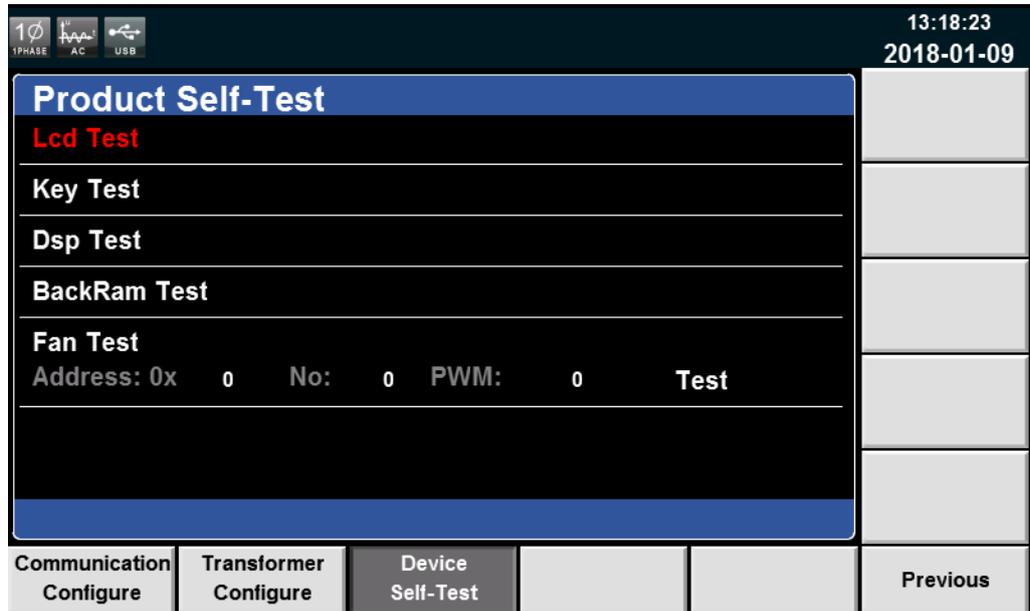
4. Press **[Enter]**, the system starts self-test. If 'LCD Checking Finish' displays on the screen, LCD has passed self-test.
