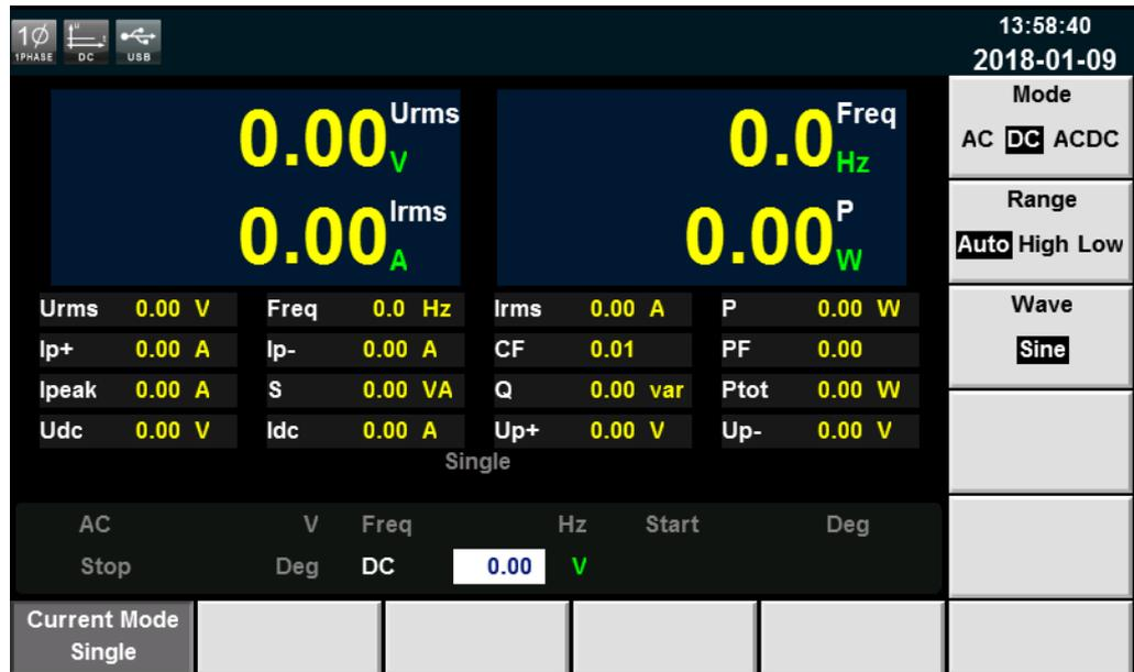
DC: DC voltage value. Setting range is different among Auto, High and Low range. Refer to 9.1 Main technical parameters for more details.
