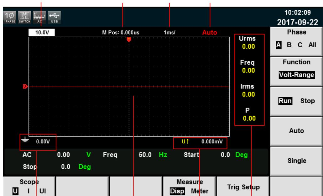
The voltage difference between ground level and point of center vertical
