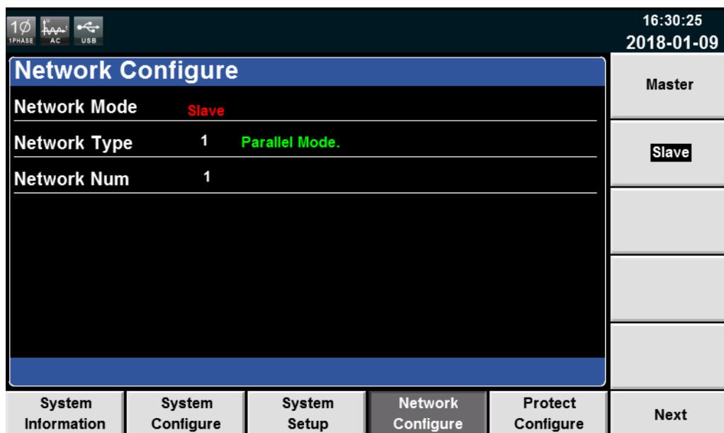
3. Press **[Esc]** to return the main interface. Power off the instrument and then power on again. (It takes about 10s to boot up the instrument.) The slave will display “SLAVE MODE! ” and the slave state is “INIT”.
