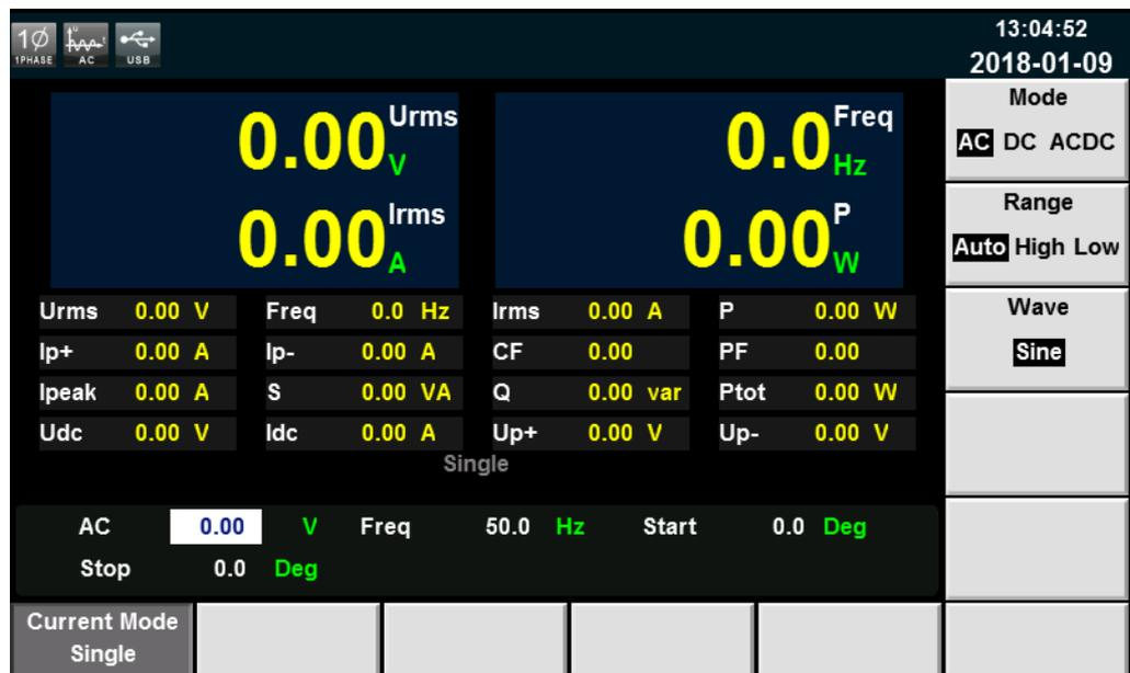
AC: AC voltage value. Setting range is different among Auto, High and Low range. Refer to 9.1 Main technical parameters for more details.
