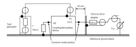
Voltage division factor RF-port to EUT-port: 150 kHz - 80 MHz: 9.5 dB  $\pm$  1dB 80 MHz - 230 MHz: 9.5 dB +3 dB / - 2 dB
