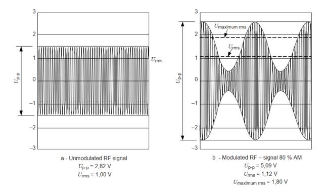
Consequently, the level of the modulated signal must be 5.1 dB higher than the test levels specified by the standard. Adding a 6dB attenuator to improve matching of the RF power amplifiers would require following amplifier output power:
